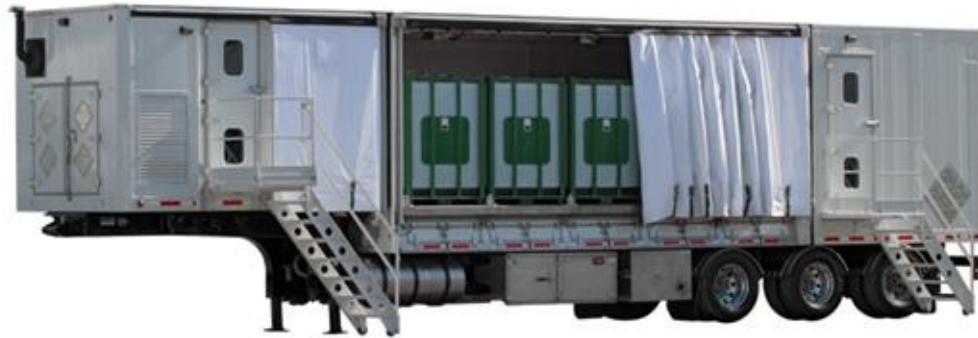
Enclosed chemical additive unit Photo courtesy of TYCROP Manufacturing Ltd.
